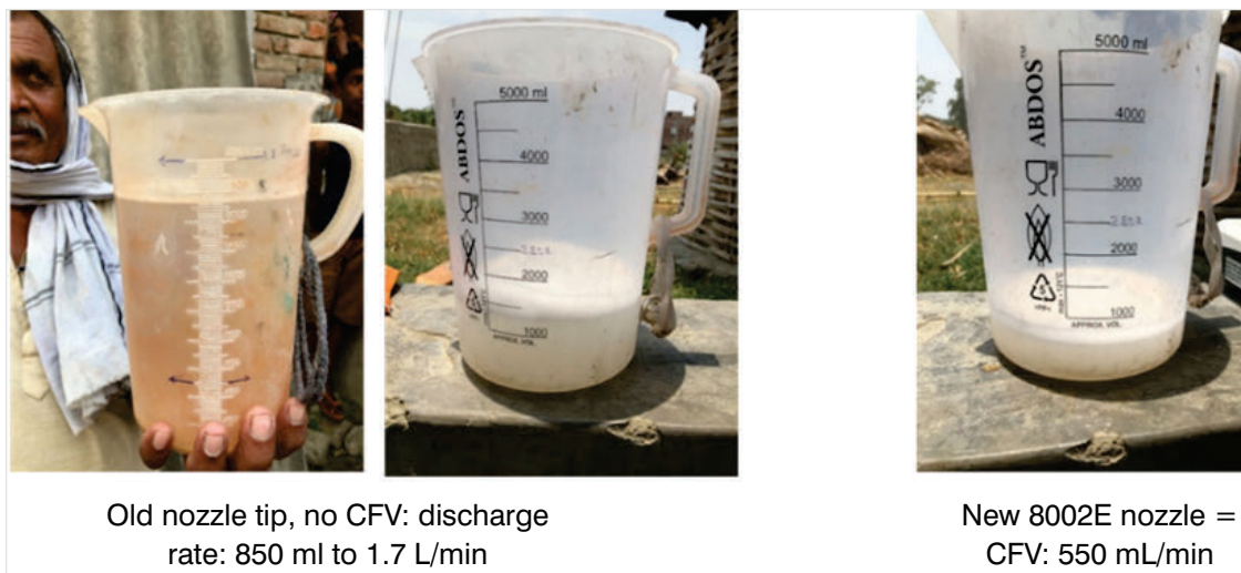
Photos 2, 3 and 4. Insecticide discharge according to the nozzle status
